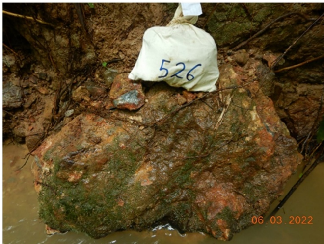
Large boulder of quartz—iron oxides-pyrite. Grab sample: 2.0 g/t Au, 26 g/t Ag, 175 ppm Cu and 10 g/t Te.
