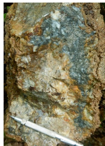
Boulder of quartz—iron oxide-pyrite. Grab sample: 1.6 g/t Au, 5 g/t Ag, 322ppm Cu and 4 g/t Te.
