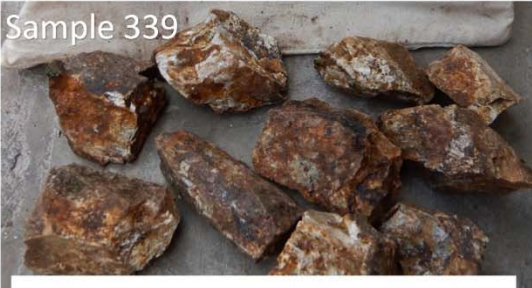
Photo 4: Sample 339. Porphyry outcrop with iron oxide veins and tenorite in fractures. 431 ppm Cu with portable XRF. Lab results are pending
