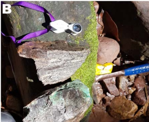
B) Cretaceous Cushabatay Formation fine sandstone with secondary copper mineralization. This sample assayed 2.5% Cu and 36 g/t Ag.
