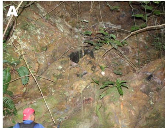
A) Typical leached gossanous sandstone outcrop anomalous in Zn and Pb. These zones typically contain 0.1-2% Zn+Pb.
