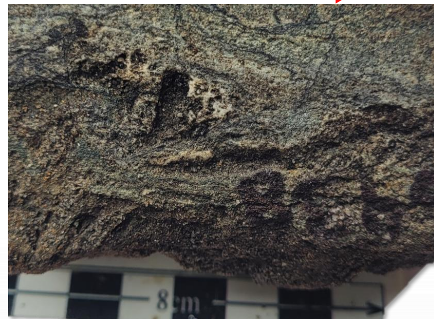
Pervasive roscoelite alteration with adularia: 1.7 m @ 23.4 g/t Au, 87 g/t Ag, 91 ppm Te
