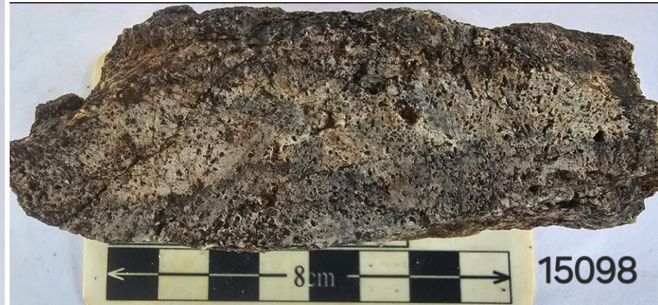
15098 Quartz with manganese oxide after rhodochrosite alteration 1.3m @ 3.6g/t Au, 27g/t Ag, 5ppm Te
