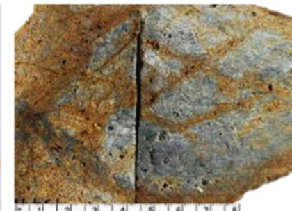
Sample 15496 2.5 m @ 0.5 g/t Au and 0.5% Ag. K-feldspar porphyry with moderate phyllic alteration..
