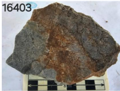
Sample 16403 2.5 m @ 1.7 g/t Au and 39 g/t Ag. K-feldspar porphyry with crackle texture and dark iron oxide patches.
