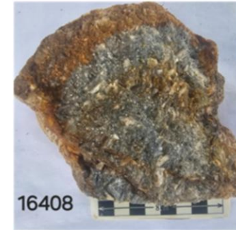
Sample 16408 3.0 m @ 5.9 g/t Au and 23 g/t Ag. Megacrystic k-feldspar porphyry with moderate phyllic alteration.
