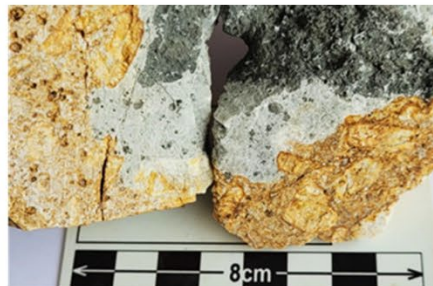
Sample 15491 3.0m @ 1.6 g/t Au and 3.1 g/t Ag. K-feldspar porphyry with moderate phyllic alteration 2% disseminated pyrite. Pyrite veinlets with grey silica and pyrite-quartz filled cavities.
