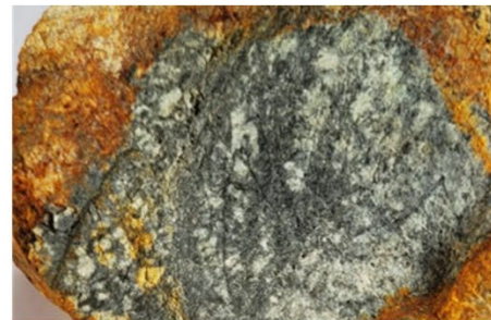
Sample 15493 3.0m @ 0.9 g/t Au and 2.8 g/t Ag. K-feldspar porphyry with moderate phyllic alteration cut by veinlets of iron oxides and silica. Spots of disseminated pyrite.
