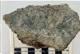
14161: mKFP; dissemination and veins with py and cpy; mal, OxFe and OxMn in fractures..
