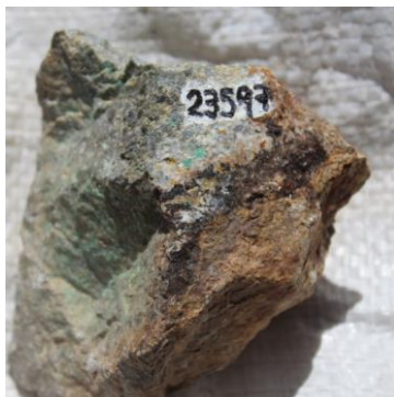
Sample 23597: Dacitic porphyry float with, moderate phyllic and weak silicification. Some malakite and iron oxides. 0.2% Cu
