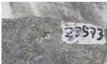
Sample 23573: Porphyry float with hydrothermal magnetite, moderate phyllic and weak argillic alteration. Dissiminated pyrite with trace chalcopyrite and covellite
