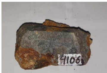
Sample 4106: porphyry float with silicification and phyllic alteration. With trace of chalcocite. 0.2 g/t Au, 0.09 % Cu
