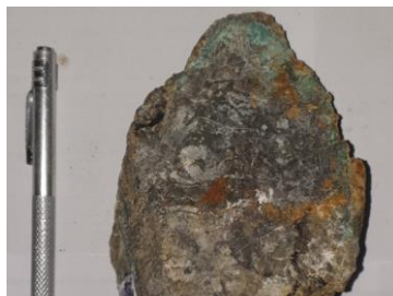
Sample 4110: strongly silicified float with secondary copper oxides. 0.12 % Cu.
