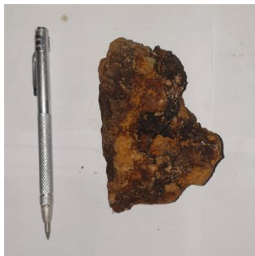
Sample 4105: hydrothermal breccia with porphyry clasts and matrix of iron oxides. 0.9 g/t Au, 0.13 % Cu, 6.7 pp, Ag 106 ppm Mo
