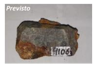
Sample 4106: porphyry float with silicfication and phyllic alteration. With trace of chalcocite. 0.2 g/t Au, 0.09 % Cu
