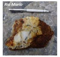
Sample 23566: hydrothermal breccia clasts of cuartzite and matrix of grounded rock. Trace chalcopyrite and copper oxides. 0.16 % Cu
