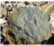
Sample 23531: Skarn float with retrograde alteration. 477 ppm Cu.
