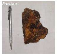
Sample 4105: hydrothermal breccia with porphyry clasts and matrix of iron oxides. 0.9 g/t Au, 0.13 % Cu, 6.7 pp, Ag 106 ppm Mo
