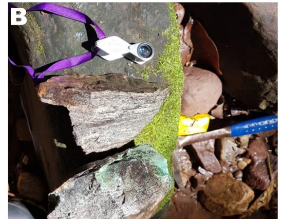
B) Cretaceous Cushabatay Formation fine sandstone with secondary copper mineralization. This sample assayed 2.5% Cu and 36 g/t Ag.
