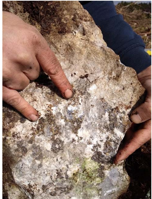
Photo 1 and 2: Coarse grained galena (silver colour – lead sulphide) and sphalerite (brown colour- zinc sulphide) hosted within calcite and limestone.
