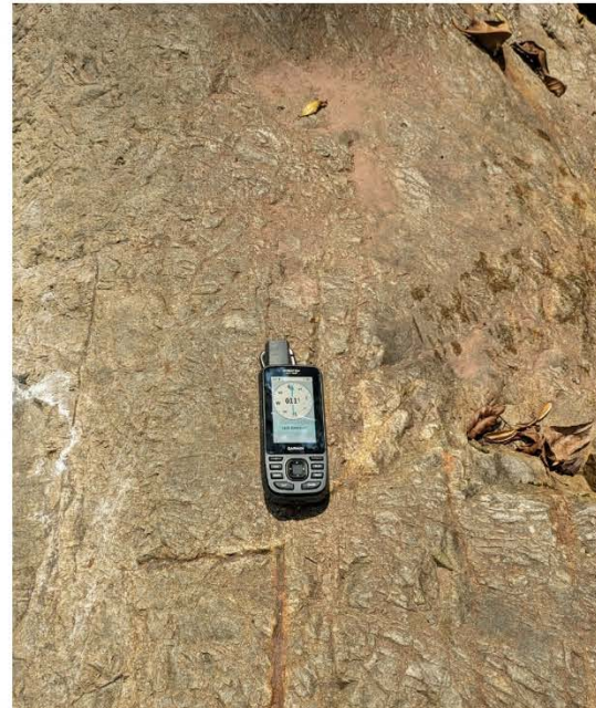
B: N-S striking quartz-pyrite veins. Three veins are visible on the photo
