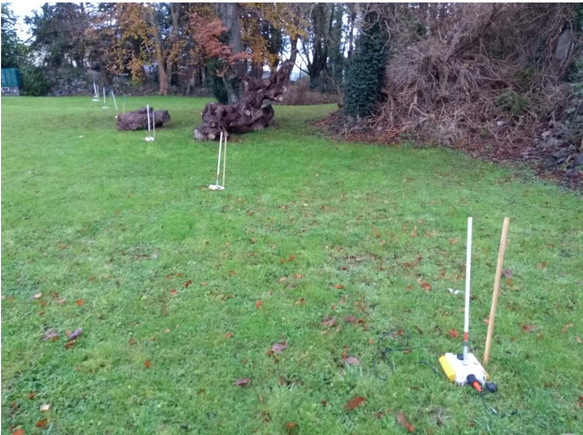
Photo 2: Wifi sensors or geophones are planted by hand on road side verges typically for periods of 2 to 5 days before being removed again.
