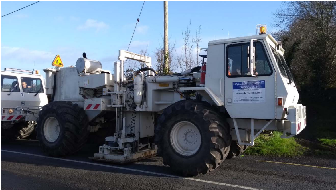
Photo 1: Two Vibroseis trucks, which stop every few metres for half a minute or so to produce the source vibrations.
